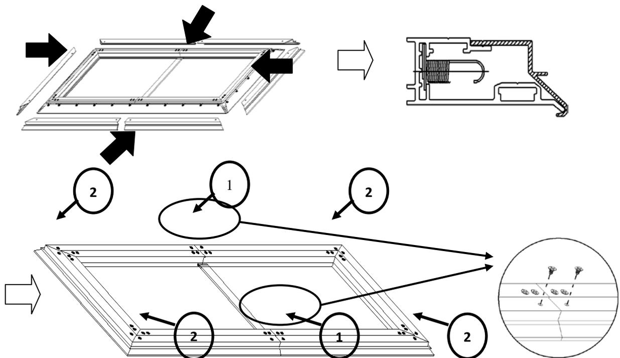
**Step 13:** Install the *angle cover (j)* on each corner of the frame and install the M4x7 screws to hold down the angle cover.
