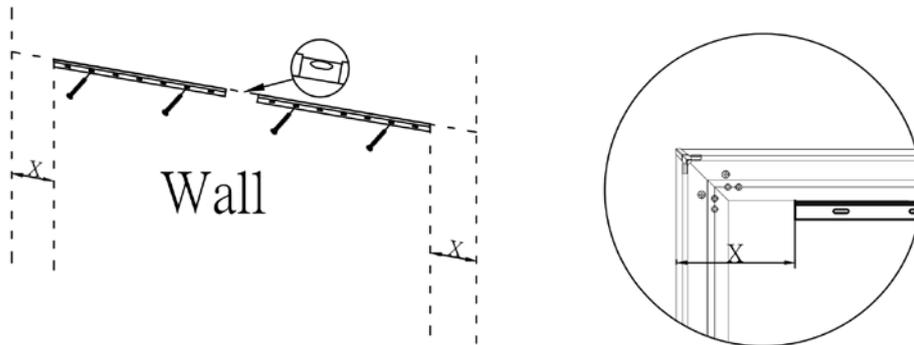
**Step 15:** Position the fixed frame screen onto the top wall brackets as shown below and push down at the center of the top of the frame to secure.
