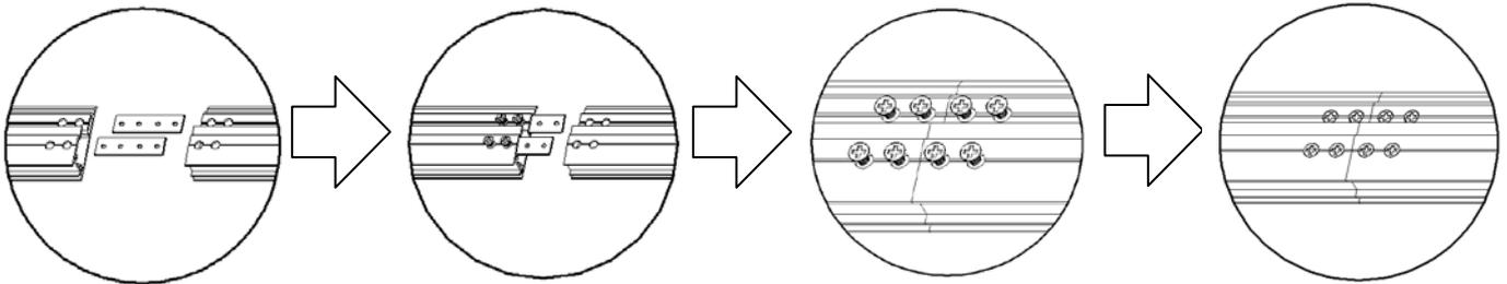
**Step 5:** Insert the *springs* (e) into the grooves of the frame. The spring's hooks should be facing the front side of the frame. For the correct amount of springs to place into the frame, please refer to the table below.
