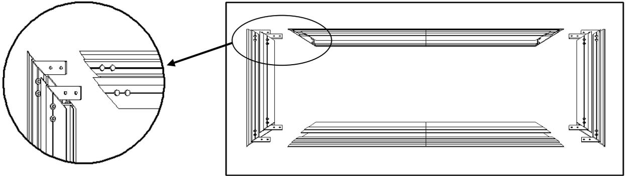
**Step 7:** Secure the elbow joints by fastening them with *M4x6 screws (c)*, 4 at each corner.
