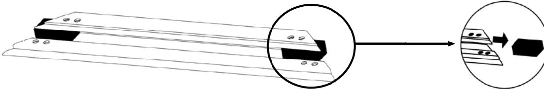
**Step 4:** Insert the *center joint* (a) connectors into *one-half of the horizontal frame* (b/c) and secure with the *M4x6 screws* (c).
