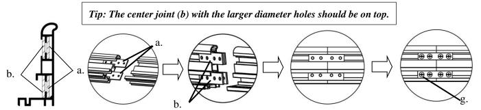
**Step 4:** Connect the *elbow joints* (*c/d*) to the top and bottom sections of the vertical frame. Once inserted, connect the vertical sections to the horizontal frame sections. Make sure all holes are in alignment and the frame pieces are flush (no gaps). They should form perfect right angles.
