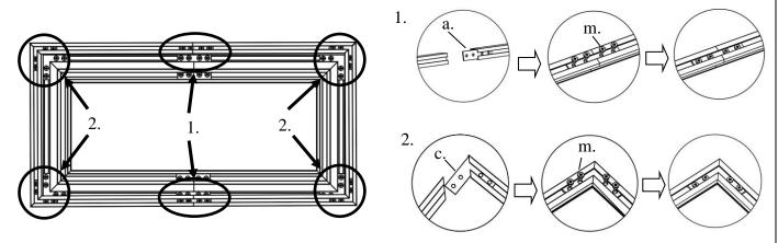
**Step 12**: Install the *angle cover* (n) on each corner of the frame as show in the illustration below.
