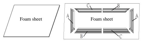
**Step 3**: Remove the foam in all frame ends before assembling the frame
