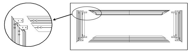
Step 6: Secure the elbow joints by fastening them with *M4x6 screws* (c), 4 at each corner.
