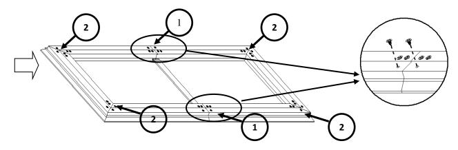
**Step 13**: Install the *angle cover (j)* on each corner of the frame and install the LED light strip to hold down the angle cover (or just use the clips if LED kit will not be installed). Then insert the *LED light clip (l)* to hold the LED light strip in place.
