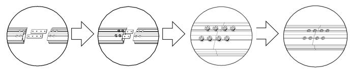
Step 5: Connect the *elbow joints* (b) to the top and bottom sections of the vertical frame. Once inserted, connect the vertical sections of the horizontal frame sections. Make sure all holes are in alignment and the frame pieces are flush (no gaps). They should form perfect right angles.
