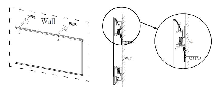
**Step 16:** With the frame slightly tilted outward; connect the bottom brackets onto the bottom groove of the frame. Then secure them by screwing onto the wall.
