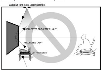
Note: Improper installation will result in light loss and produce a dark image. This is due to the projector's light reflecting in the wrong direction.
