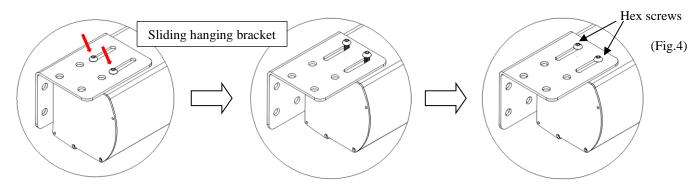
**Note:** It is the responsibility of the installer to select the appropriate mounting hardware and assure the mounting surface is of adequate strength to safely install the screen. The screw hole of sliding hanging bracket is M10 (Fig. 5).
