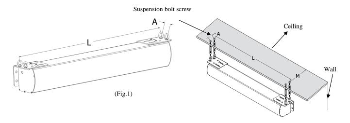
2. Next, attach the *M10 Suspended turnbuckle hooks* (A) to all four *M10 eyebolts* (B) installed on the brackets (A/B/C/D). Then hang the screen to the *suspension bolt hooks* installed on your ceiling.
