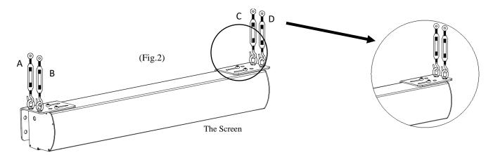
3. After the installation is complete, if the screen is not leveled, you can adjust the height of the suspended hooks to level the screen. Below are the adjustment methods for the suspended hooks. The maximum and minimum adjustable lengths are shown in Fig 3, illustration 3 and 4.
