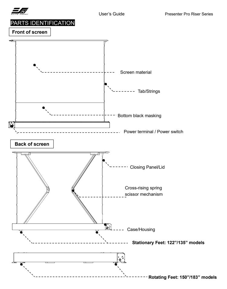
Note: Please always store the screen flat horizontally. Never store the screen in a vertical position as it will permanently damage the screen's structure, shift the material, and cause wrinkles/folds which will void the warranty.
