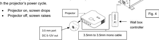
5. Wireless 5-12 volt trigger (Fig.5): Requires a 3.5mm to 3.5mm mono cable (Not included).
