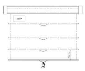
2. To retract the screen, simply pull the screen downward from the handle or lanyard more than 2 inches (5cm) and retract the screen back releasing it up gently. **DO NOT let go of the handle until fully retracted in the housing.**
