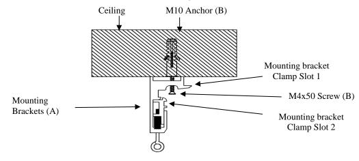
3. Insert the and attach the *Top Case Slot A* to the *Top Clamp Slot 1*, then secure it by pushing and clicking it in the *Bottom Case Slot B* to *Bottom Clamp Slot 2*. Make sure the case slots are securely attached to the mounting brackets.
