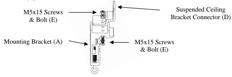
3. Insert chains (not included) through the loopholes of the Suspended Ceiling Bracket Connector (D).
