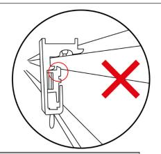
**CAUTION:** THE WALL BRACKET MUST BE SECURELY LATCHED IN THE CASE SLOTS TO PREVENT THE CASE FROM FALLING OFF.
