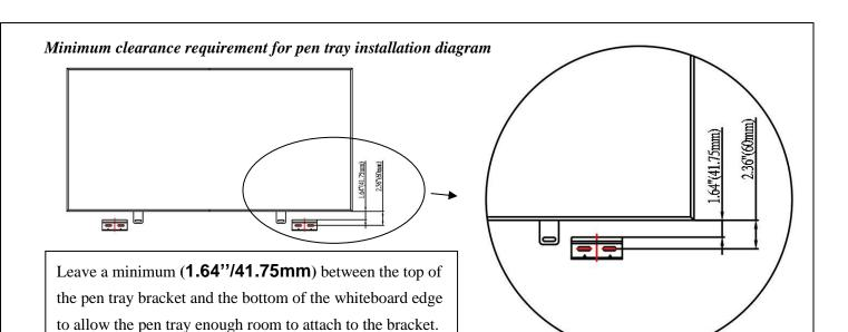
Step 5: Attach the pen tray on the tray hanging bracket as shown in the steps below.
