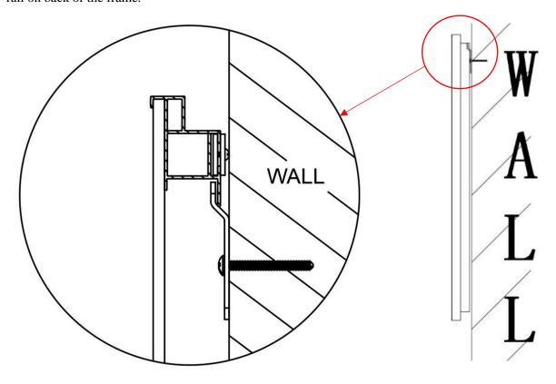
Step 3: Next, attach the *Bottom Hanging Brackets* (d) to the bottom frame, again making sure the lip of the bracket inserts in the rail. Then, drill holes according to the holes on the bottom brackets to insert and screw the wall screws to secure the bottom hanging brackets to the wall.
