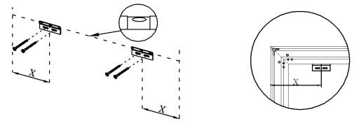
**Step 15**: Position the fixed frame screen onto the top wall brackets as shown below and push down at the center of the top of the frame to secure.
