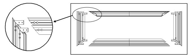
Step 6: Secure the elbow joints by fastening them with *M4x6 screws* (c), 4 at each corner.
