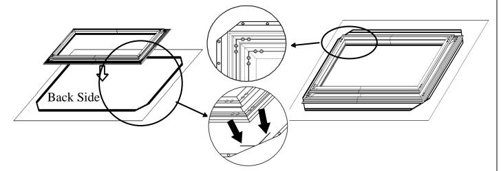
Step 10: With one end of the spring and secure inside the groove of the frame, use the spring hook (d) to attach the spring to the hole located on the screen material's outer edge in the following order.
