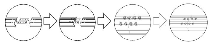
**Step 5:** Connect the *elbow joints (b)* to the top and bottom sections of the vertical frame. Once inserted, connect the vertical sections of the horizontal frame sections. Make sure all holes are in alignment and the frame pieces are flush (no gaps). They should form perfect right angles.
