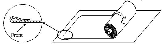
**Step 8:** Insert the *fiberglass rods (n)* through the openings. The longer rods are used on the vertical edges of the screen material, and the shorter rods are used on the horizontal edges, as shown below.
