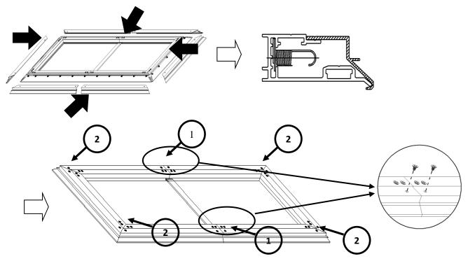
Step 13: Install the *angle cover(j)* on each corner of the frame and install the LED light strip to hold down the angle cover.
