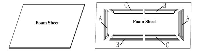
Step 3: Remove the foam on all frame ends before assembling the frame.
