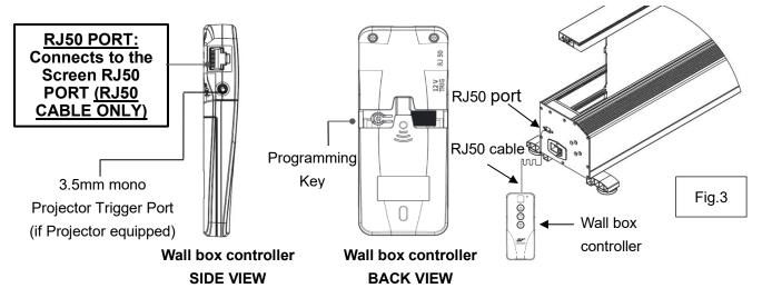
4. Wired 5-12 volt trigger (Fig.4): Requires a 3.5mm to 3.5mm mono cable (Not included)
