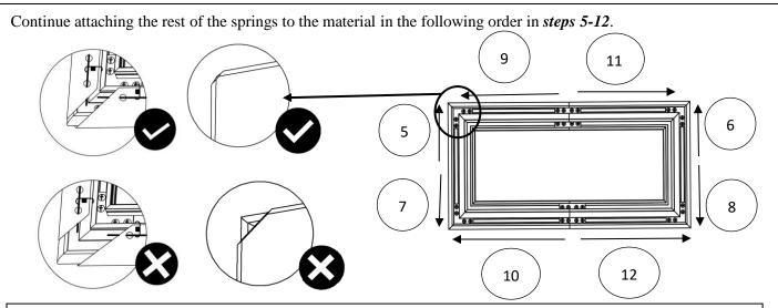
To avoid ripples forming in the material it is imperative that all of the corners are properly wrapped around the edges as illustrated in the check mark diagrams.
