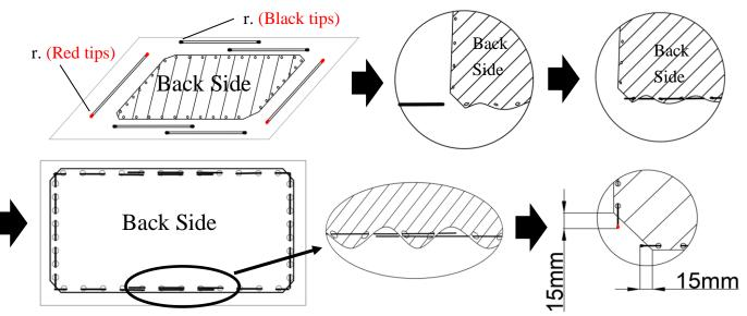
**Step 8:** Carefully and gently place the assembled frame on top of the screen material in the marked areas as shown below. Make sure to not allow the angle edge of the frame to come in direct contact with the screen material to avoid puncturing it.
