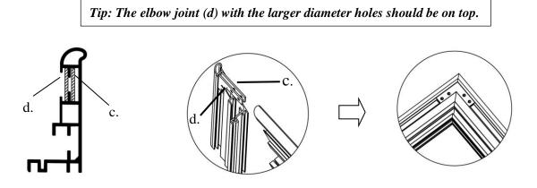
Step 5: Secure the elbow joints by fastening them with M4x7 screws (g), 4 at each corner.
