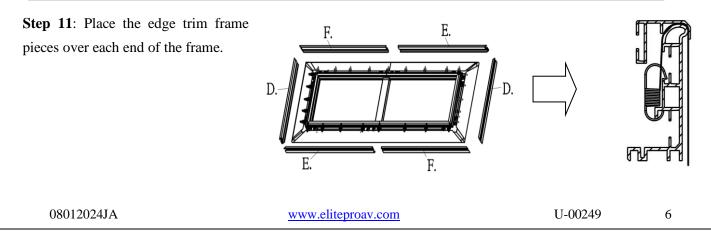
Connect edge trim frames (e/f) together using the *Center Joints- M4(a)* and secure with four of the *M4x4 Screws (m)* as shown in *Step 1*. Repeat for other side.
