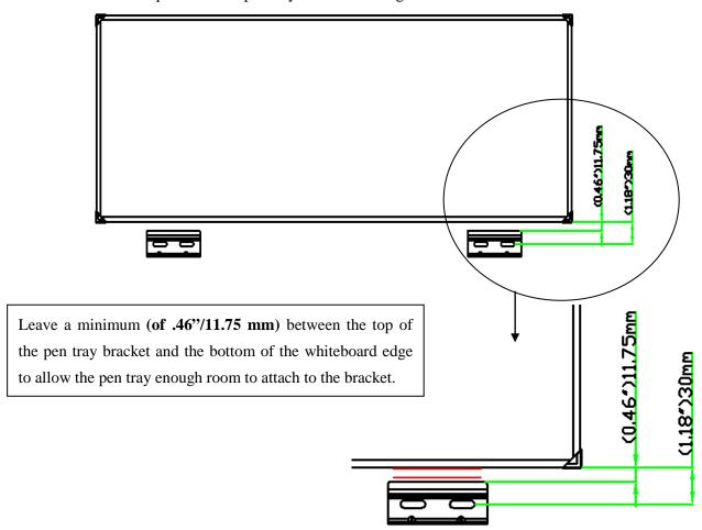
**Step 5:** Attach the pen tray on the tray hanging bracket as shown in the steps below.
