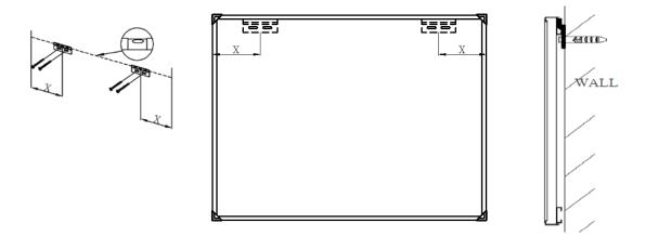
**Step 2:** Hang the WhiteBoardScreen on the *Top Hanging Brackets*, making sure the top lip inserts into the rail on back of the frame.
