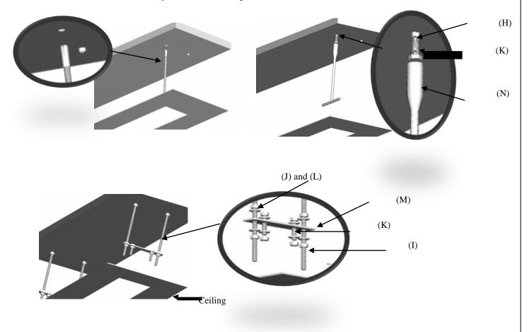
4. Push the screen up into the space. Use the threaded rods (I) to attach the screen assembly to the ceiling. The hexagonal screws (K) will connect the screen to the rest of the assembly. Once firmly in place, use the nuts (J) to ensure a firm connection. Use the socket wrench (N) to make sure that the bolts are firmly tightened.
