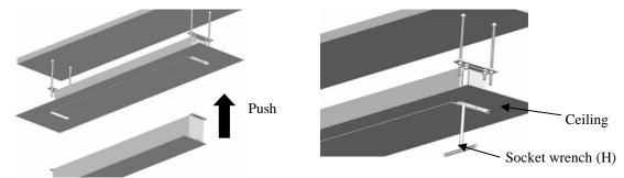
5. Install plastic cover panel (N) to complete the installation.
