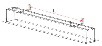
2. Mark the location of where the screen will be installed according to the distance (L) and then secure the bolt to the ceiling.
