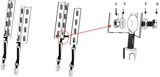
2. Attach the Suspension Bar J-Hook (G)to the Hanging Bracket (C) as shown in figure below. Install the Suspension Bars (D) to your ceiling according to their distance.
