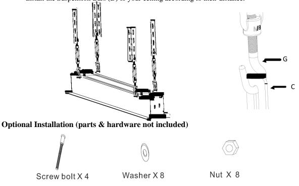
1. Place the Hanging Bracket (C) in the desired location on the screen's housing and measure the distance as shown below. (L = Distance)
