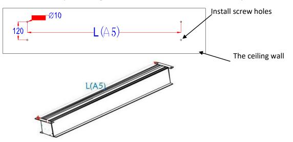
3. The expanding bolts (H) mount into thick wood beams, stone or concrete and will support the screen. Use the Socket wrench (N) to attach the hexagonal screws (K). The expanding bolts should be firmly tightened and tested to make sure that they will hold the weight of the screen.
