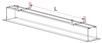
2. Mark the location of where the screen will be installed according to the distance (L) and then secure the bolt to the ceiling.
