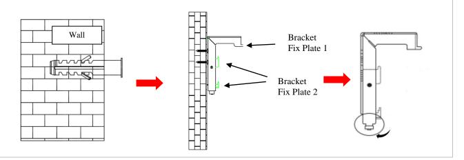
3. Attach the screen to the **Brackets** (A) by inserting the top of the case to Fix Plate 1 and securing the back of the case to Fix Plate 2.
