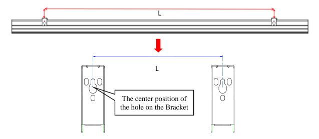
2. Drill the holes and install the **Brackets** (**A**) on the wall with the **M5.5 screws** (**D**). Make sure to level the bracket using a carpenter's level. Then loosen the screw under the **Bracket** (**A**) by turning it counterclockwise. **If no wood studs are available, use the anchors on drywalls that are at least ½" thick.**
