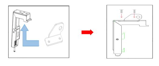
**3.** Attach the screen to the **Brackets** (A) by inserting the top of the case to **Fix Plate 1** and securing the back of the case to **Fix Plate 2**.
