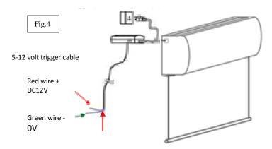
**6.** <u>Wireless 5-12 volt trigger</u> (**Item F, Fig 5**): The RF remote control serves as a dual purpose, independently as a handheld remote control, or as a Wireless 5-12 volt trigger using the trigger cable. The radio frequency technology can be programmed to send a wireless signal that synchronizes screen drop & rise with the projector's power cycle.
