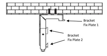
4. Attach the screen to the **Bracket (A)** by inserting the top of the case to **Fix Plate 1** and securing the back of the case to **Fix Plate 2**.
