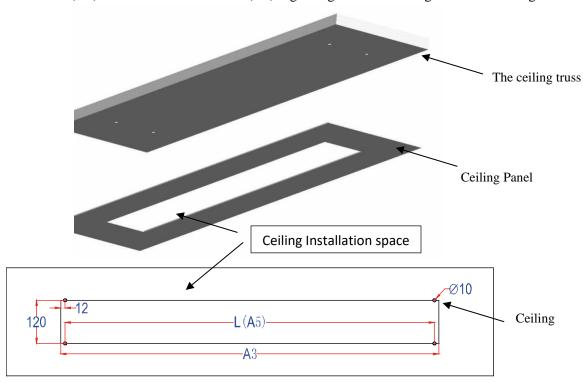
2. Drill 4 holes in the ceiling that correspond with the attachments on the various casing sizes.
