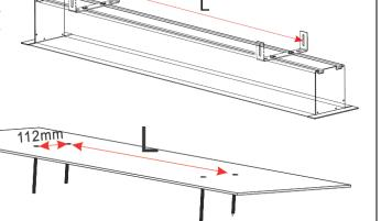
2. Mark the location of where the screen will be installed according to the distance (L) and then secure the bolt to the ceiling.
