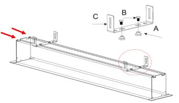
2. Place the Suspension Bar (D) on the Hanging Bracket (C) and align with the hole as shown below. Secure the Suspension Bar (D) with the Hex Screw (B), Washer (E) and the Hex Nut (F). Install the Suspension Bars (D) to your ceiling according to their distance.
